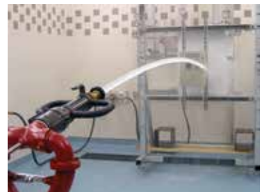
iQpump Micro NEMA-4X Washdown Test
